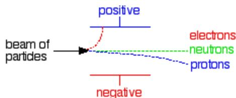
If beams of the three particles, all with the same speed, are passed between two electrically charged plates:
